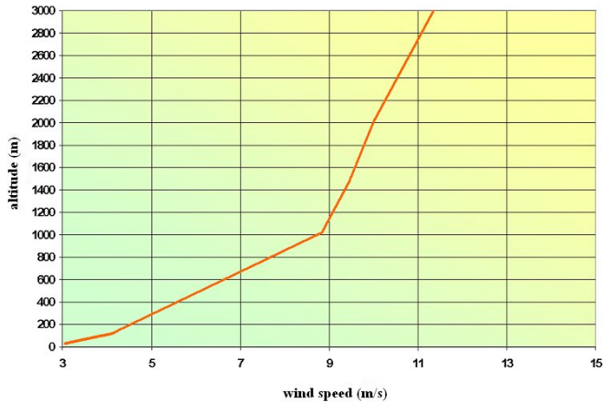
Fig. 2. Variation in the wind speed, as a function of the altitude, based on the average European wind speed (3 m/s at ground level).
